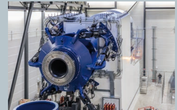
Front-end view of the wind-load unit of the LORC HALT test facility.
