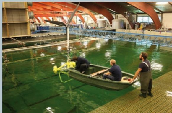
In the wave basin at DHI, researchers from DTU are mounting a model of a 10 MW turbine on a model of the Stiesdal TetraSpar floating.
