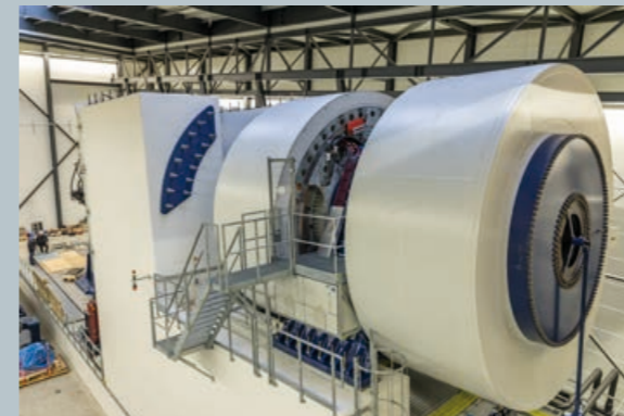
The 13MW drive-line of the LORC HALT test facility.
